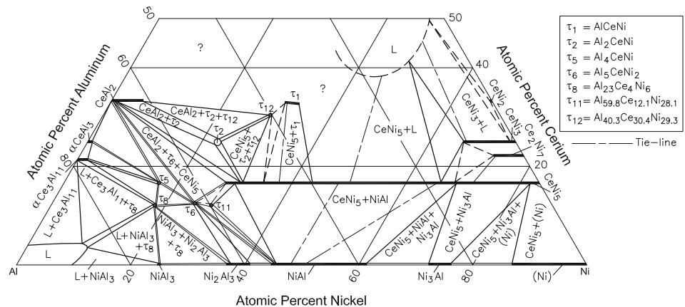
**Fig. 1** Al-Ce-Ni isothermal section at 800 °C for Ce-lean alloys [2008Tan]
