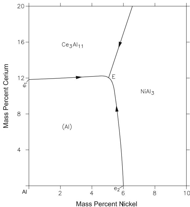
**Fig. 2** Al-Ce-Ni liquidus projection near the Al corner [1996Bel]
